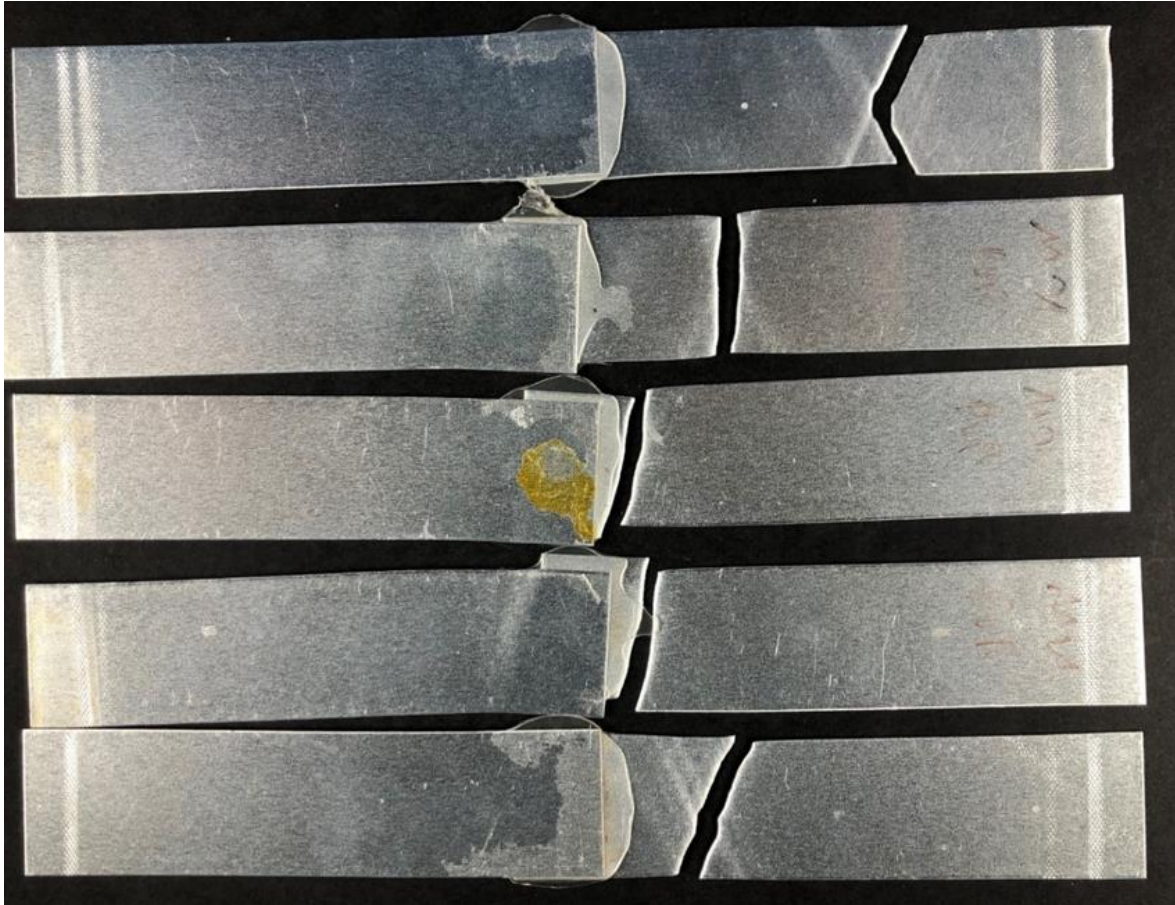
Figure S18. Aluminum plates after lap shear test of 4D.
